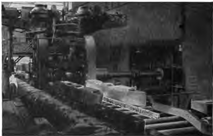
FIG. 194.—Blooming Mill Showing Steel Ingot Reduced to Bloom.
